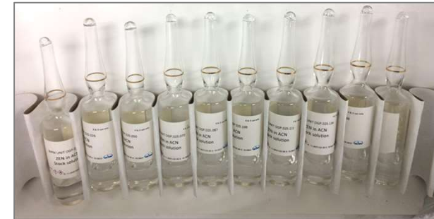
Figure 2. ZEN stock solution OGP.025 Concentration 130.1 \pm 2.2 \mu\text{g/g} ( k=2 )
